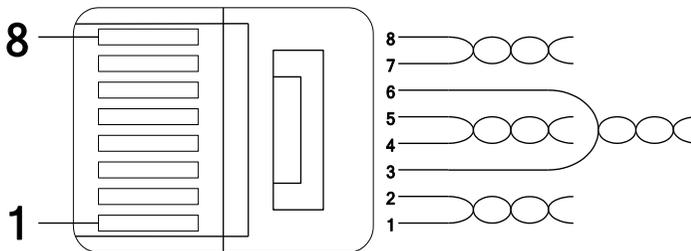
\*\* Wires connected to pin #1 and pin #2 must be twisted.
